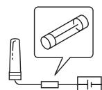
To protect the power supply and other internal circuitry, be sure to install an external fuse.
